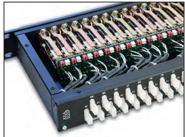
488 Series Programmable patchbay shown with dust cover removed, exposing red and white internal programming shunts.
