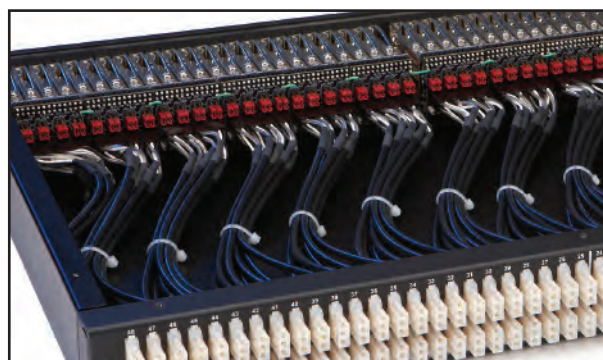
968 Series Programmable patchbay shown with dust cover removed, exposing red and white internal programming shunts.
